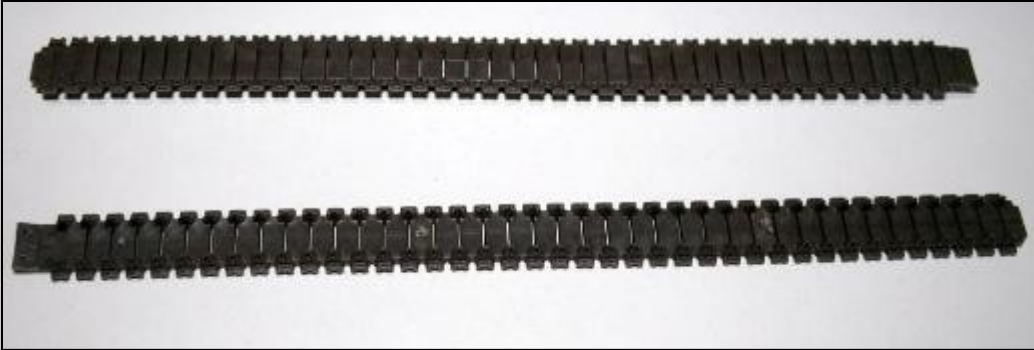
Here are the T51 block tracks used on the Sherman III. Cementing these two pieces together will make one track. Photograph by Roderick Bell .
