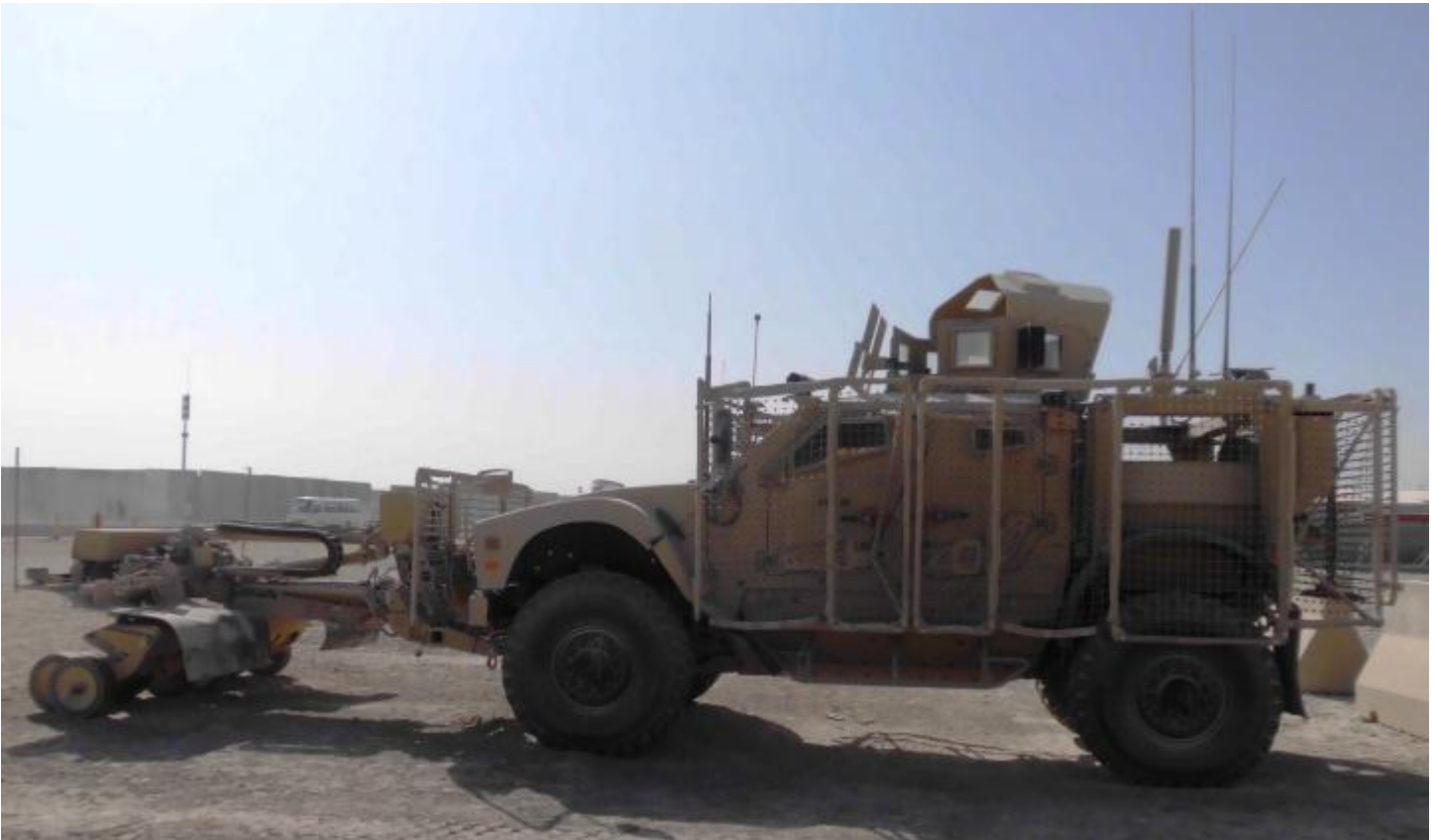
MRAP-ATV Minesweeper in Kandahar Airfield, Afghanistan. Note the anti-RPG cage. Photo taken January 8, 2012 by Michael Burns.
