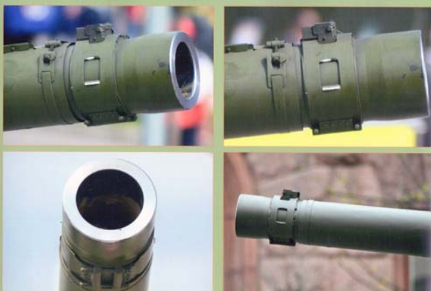
The current armament of the T-14 "Armata" is the 100mm 2A46 tank gun, which does not feature a bore evacuator but has a bypass valve built into the breech and is constructed of a new grade of steel providing significant increase in gun barrel pressure loading capability. Note the muzzle reference system sensor (star) and immediately behind the turret muzzle sensor.
