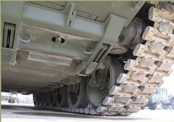
Lower glows, and track fitted with rubber pads for road travel.
