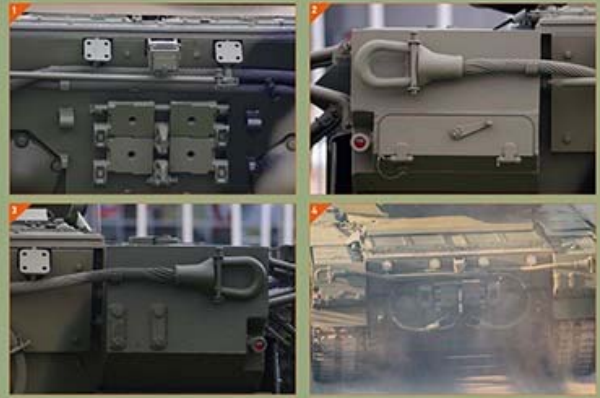
Dark track links stored on the rear armor plate. Two low cables stored on the rear armor plate. Two cables clamped to the rear armor plate. Two cables and one of four fuel-drum bracket mounting points.
