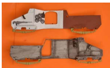
Sidewalls before (top) and after (bottom) weathering.
